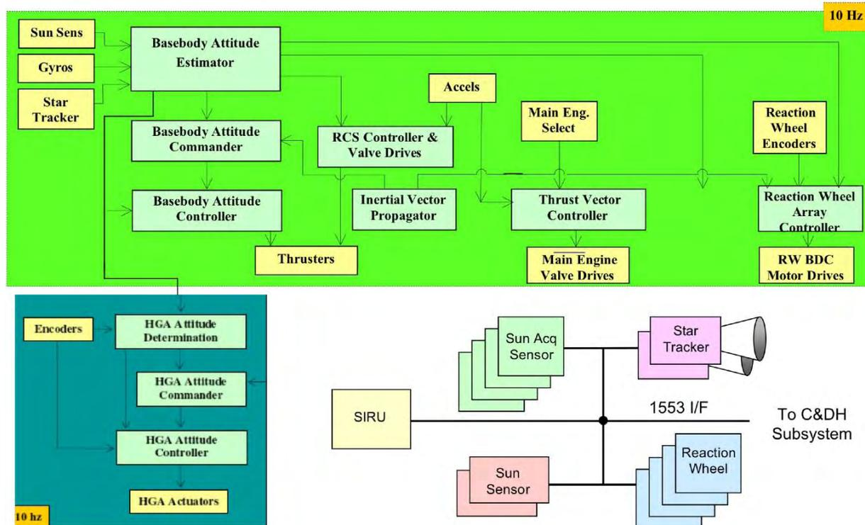
Figure 4.4-13. AACS Functional Block Diagram
