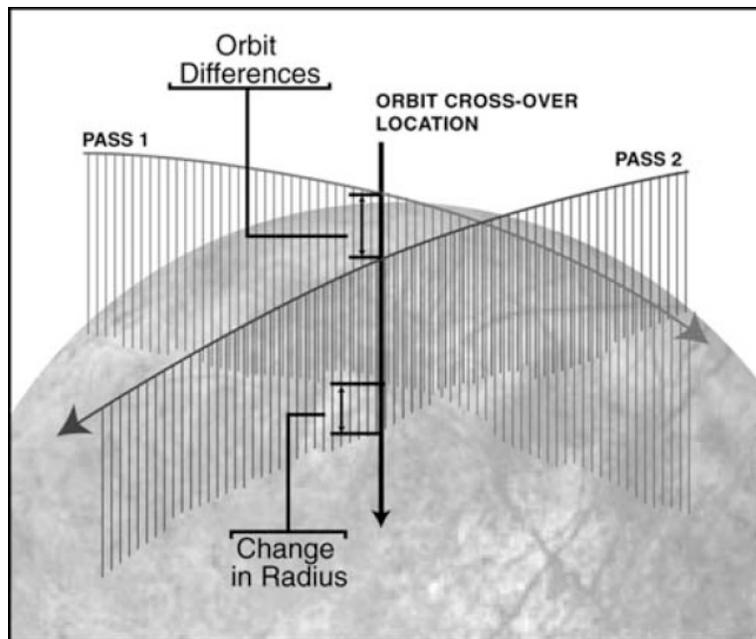
**Figure 2.3-3. Illustration of the cross-over technique.** Actual change in radius of Europa due to tidal and librational motions is determined by measuring altitude from the spacecraft to the surface, and by accounting for the distance of the spacecraft from the center of mass by means of Doppler tracking [Wahr et al. 2006].
