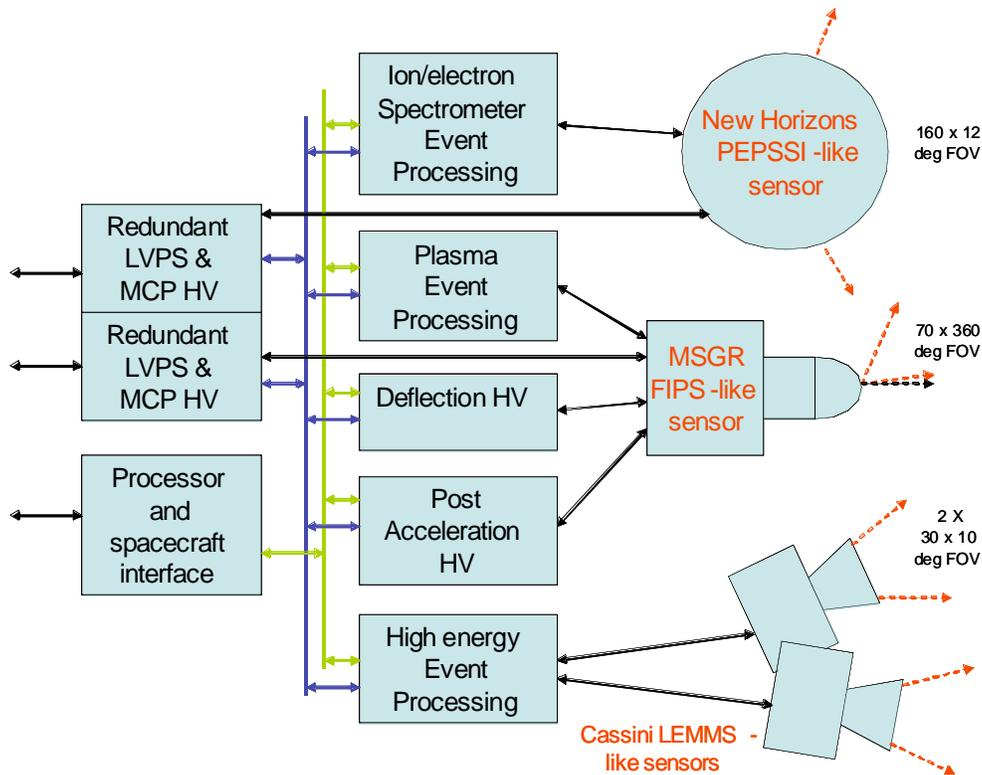
**Figure 4.2-9. Particle and Plasma Instrument (PPI) block diagram.**
