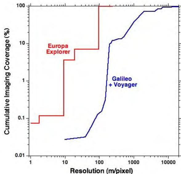
**Figure 2.3-6. Cumulative imaging coverage of Europa’s surface as a function of imaging resolution, illustrating the 1–2 orders of magnitude improvement of planned EE imaging coverage relative to that from Voyager and Galileo combined. Unlike the opportunistic coverage obtained from earlier fly-bys, EE’s deliberate imaging coverage from orbit will be in discrete resolution steps.**
