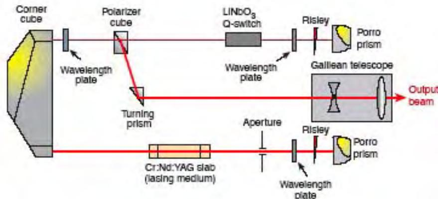
**Figure 4.2-4.** Optical Schematic from the NEAR Laser Rangefinder. NLR laser resonator cavity configuration is a polarization-coupled U-shaped cavity design. The Cr,Nd:YAG zigzag slab is side-pumped by a diode laser array to optimize conversion efficiency [Cole 1998].
