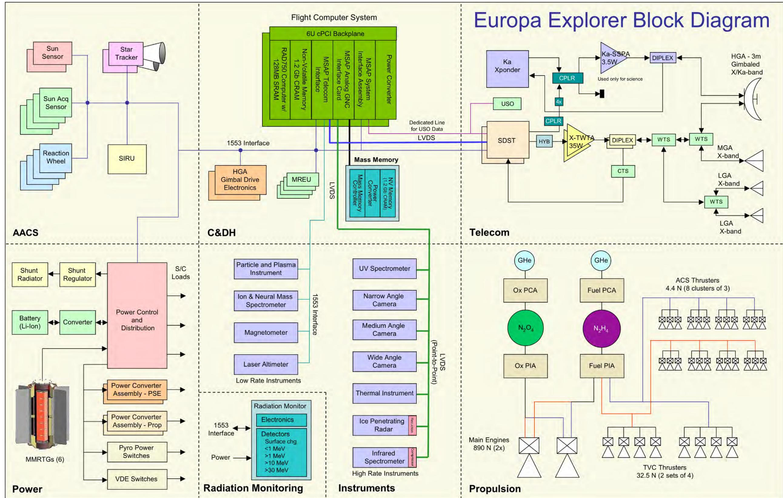
maintenance  $\Delta V$  maneuvers are performed using the same 4.4 N monopropellant thrusters that are used for attitude control. The total capability of the propulsion system, using the main engine and the smaller thrusters, is 2755 m/s.
